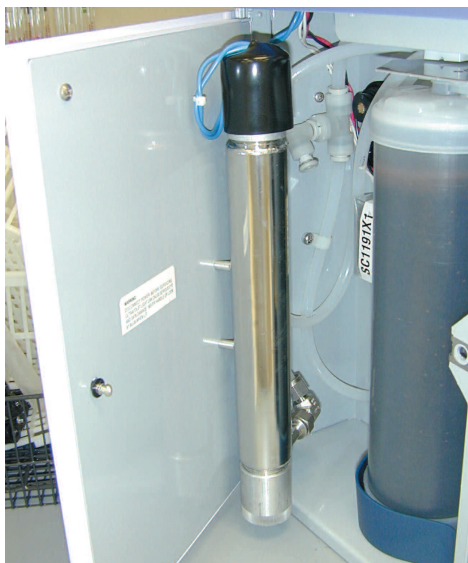
Figure 17: UV Lamp Installation
